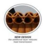
Figure 5. Hollow bamboo as the additional layer to reduce heat transmission in *Teda wewa* (Source: Authors)
